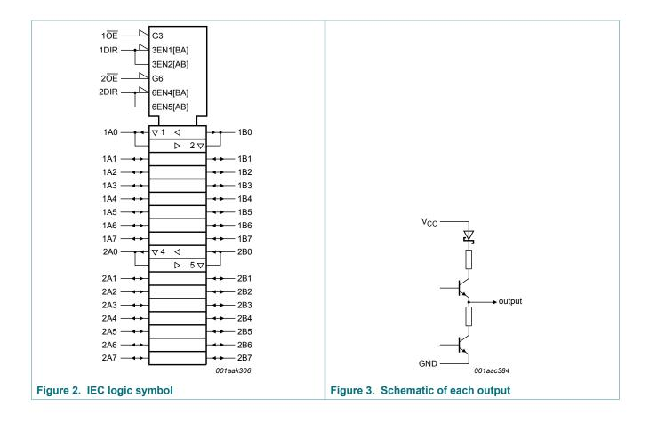
16-bit bus transceiver with 30  $\Omega$  series termination resistors; 3-state
